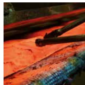
Brazing as the permanent connection of tungsten carbide and steel
