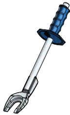
▪ BZ42 Bit extractor for BSH on BC-Series
